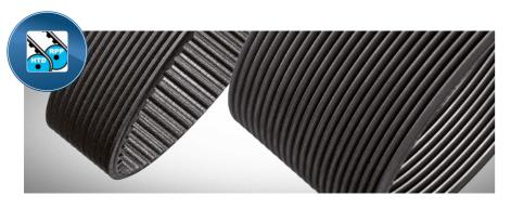
The **optibelt OMEGA RB** timing belt with additional ribbed PK belt section on the top surface of the belt is perfect for use in mills where the back pulley has a reversible direction and slipping is necessary when the drive blocks.
